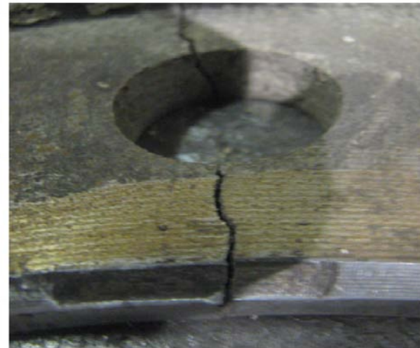
Installed on Incorrect Hub
